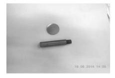
Fig.1: Work piece and Electrode
