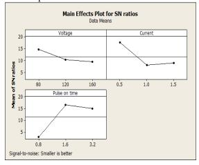
Fig.1: SN ratio plot for surface roughness
